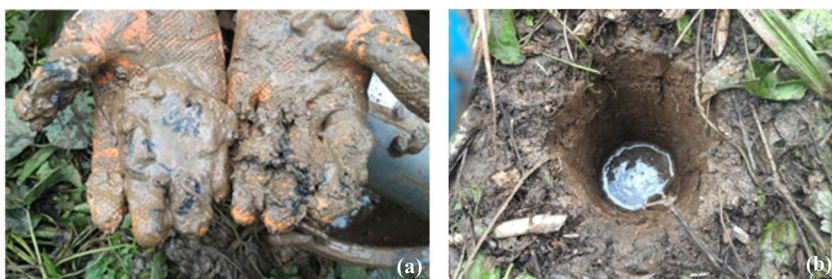
Figure 4. (a) The unnaturally very fine black particles in KT3P samples similar to the mine tailings from the ore flotation process, and (b) KT3P filled with water.
