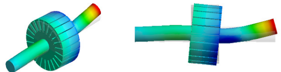
2 nd Bending Mode (4,505 Hz)
