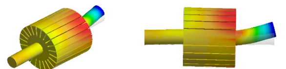
2 nd Bending Mode (4,514 Hz)
