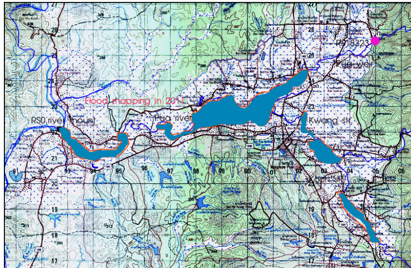
Fig. 15 Flood delineation and mapping in 2011 in the Pua and Kwang, drawn on the topographic map interpreted from the result of HEC-RAS
