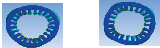
Stator 3 rd Bending Mode (16,953 Hz)
