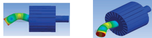
Rotor 1 st Bending Mode – 17,730 Hz
