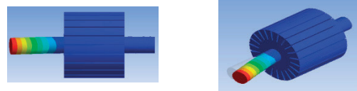
Rotor 1 st Sway Mode – 3,470 Hz
