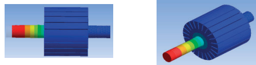
Rotor 1 st Flexible Mode – 19,723 Hz
