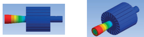
Rotor Rotational Modes – 14,098 Hz
